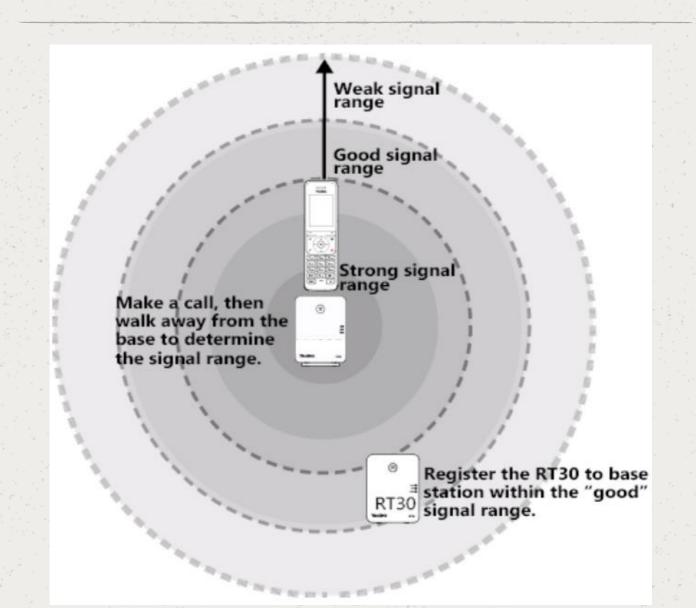
The optimum location for the repeater is as far from the base as possible while still maintaining a good signal, or just inside the location where the noise became noticeable.
