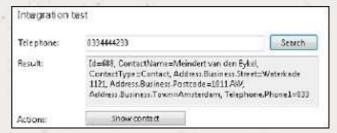
The test area results should look similar to the results showing in the image here. If the test does not work, go to the 'Log' page of configuration and turn on logging, then do the test again and see if there are any errors in the log.
